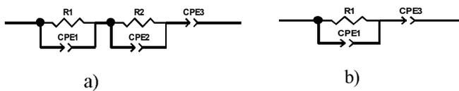
Fig. 3. Equivalent impedance circuits of cell with  $\text{Pb}_{1-x}\text{Sm}_x\text{SnF}_{4+x}$  at 293 (a) and 473 K (b)
