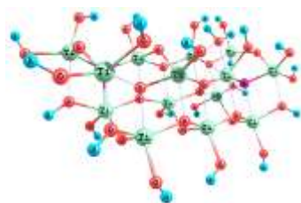
Fig. Adsorption of water molecules on the N-doped anatase face (001) with an oxygen vacancy
