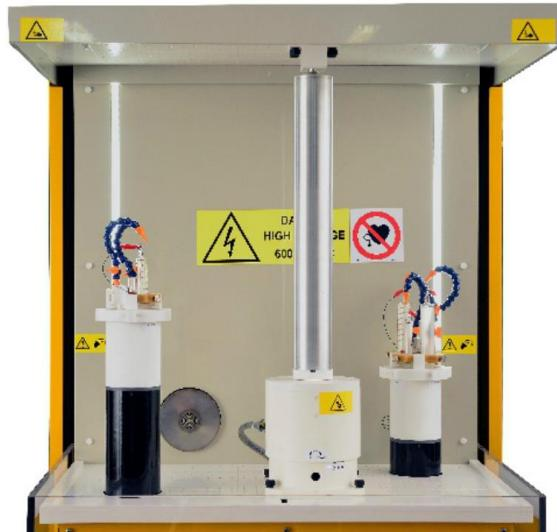
Spinning of membranes at voltages up to 60000V
