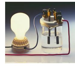
▲ A solution of sodium chloride in water conducts electricity, allowing the bulb to light.
