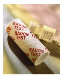
▲ Radon gas can be detected and measured by this home detection kit.
