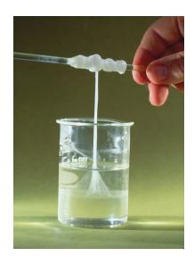
▲ Nylon being pulled from the interface between adipic acid and hexamethylenediamine.
