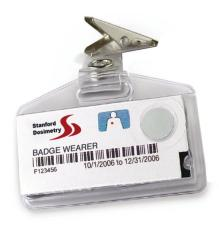
▲ This photographic film badge is a common device for monitoring radiation exposure.
