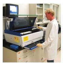
▲ Radiation is conveniently detected and measured using this scintillation counter, which electronically counts the flashes produced when radiation strikes a phosphor.
