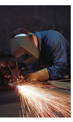
▲ Acetylene is frequently used for welding metal because it burns with such a hot flame.
