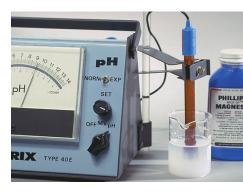
▲ **FIGURE 10.4** Using a pH meter to obtain an accurate reading of pH. Is milk of magnesia acidic or basic?
