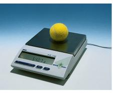
▲ The tennis ball weighs 54.07 g on this common laboratory balance, which is capable of determining mass to about 0.01 g.
