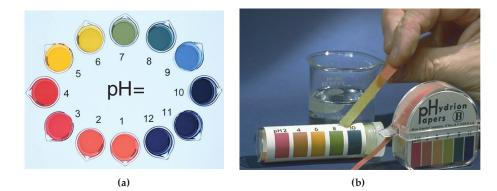
▲ **FIGURE 10.3 Finding pH.** (a) The color of universal indicator in solutions of known pH from 1 to 12. (b) Testing pH with a paper strip. Comparing the color of the strip with the code on the package gives the approximate pH.
