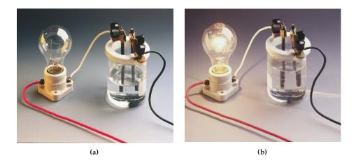
▲ FIGURE 9.8 A simple demonstration shows that electricity can flow through a solution of ions. (a) With pure water in the beaker, the circuit is incomplete, no electricity flows, and the bulb does not light. (b) With a concentrated NaCl solution in the beaker, the circuit is complete, electricity flows, and the light bulb glows.
