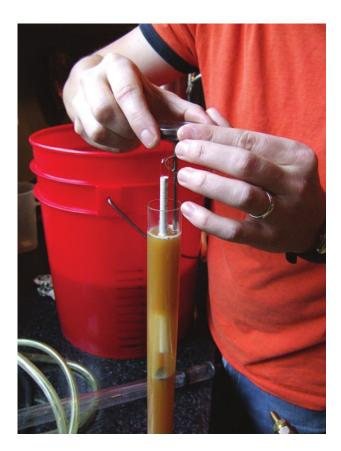
▲ The amount of fermentation that has taken place in the wine can be measured with a hydrometer.
