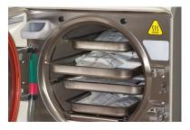
▲ Medical instruments are sterilized in this autoclave by heating them with water at high pressure.
