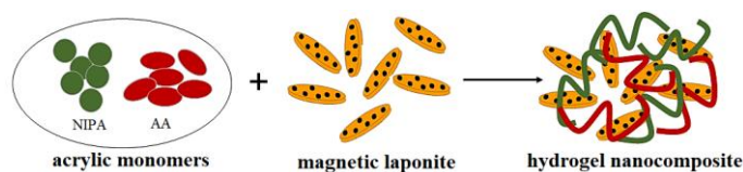
Fig. Schematic diagram for the synthesis of hydrogel nanocomposite based on magnetite-laponite
