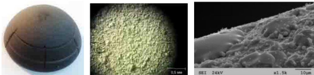
Fig. Photos of the sapphire insert surface with a titanium coating at different magnifications
