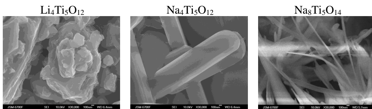
Fig. Scanning electron micrographs of alkali metal titanates obtained at the same magnification
