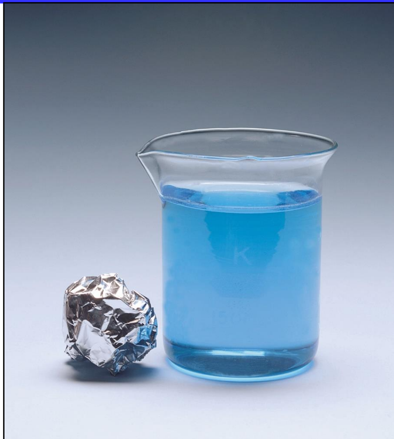
(a): Placing Al in \text{CuCl}_2 dissolved in \text{H}_2\text{O} forms \text{Cu}^{2+} ions
