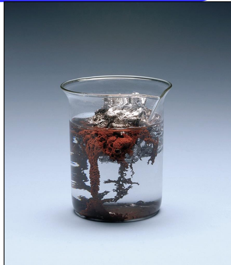
(b): \text{Cu}^{2+} in solution is reduced to Cu metal
