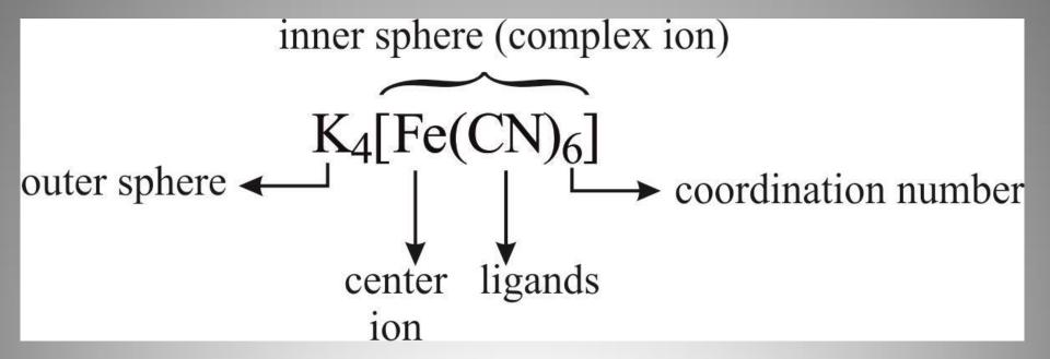
According to the coordination theory, in the centre of a molecule of a coordination compound the central atom (ion) is situated.
